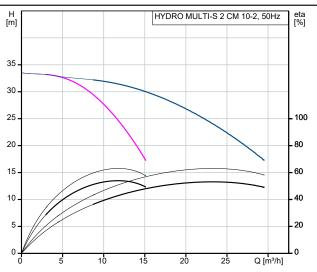
Losses in fittings and valves not included Pumped liquid = Water Liquid temperature during operation = 20 °C Density = 998.2 kg/m³
